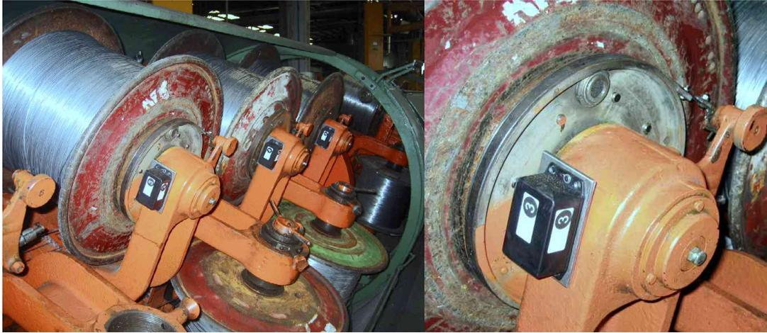
The usual wire break detectors based on the control of rotation of the reel can not be installed in machines having no sliding contacts brushes.
